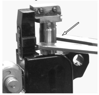
Figure 10. Pin Wrench Unscrewing Gland
