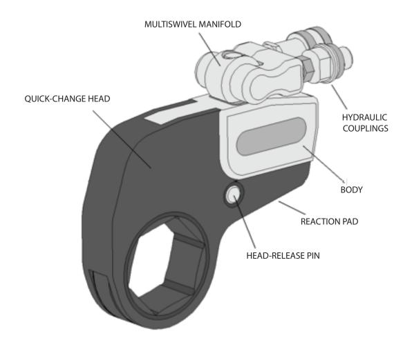
Figure 1. TWLC Hydraulic Torque Wrench
