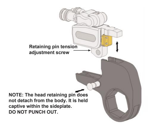
Figure 2. Body and Drive Head Removal and Attachment
