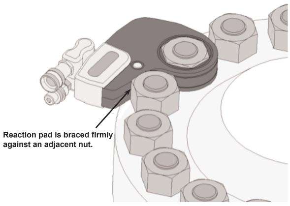
Figure 4. Correct Positioning of the Hydraulic Torque Wrench
