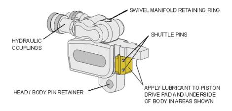
Figure 5. TWLC Hydraulic Torque Wrench Maintenance
