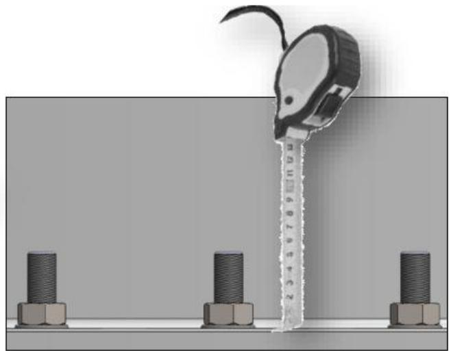
Ensure that there is enough engagement length between the bolt and the tensioner, but it must be less than the maximum allowed by the tensioner.
