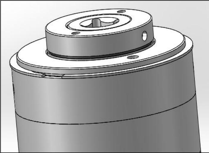
The tensioner stroke cannot exceed its maximum value. Check the common specification table of HTE tensioner for stroke parameters. When the maximum stroke is reached, the warning line can also be seen on the piston. If the maximum pressure is reached on this line, abandon the tension cycle. Tighten the nut, release the pressure, and pressurize again.
