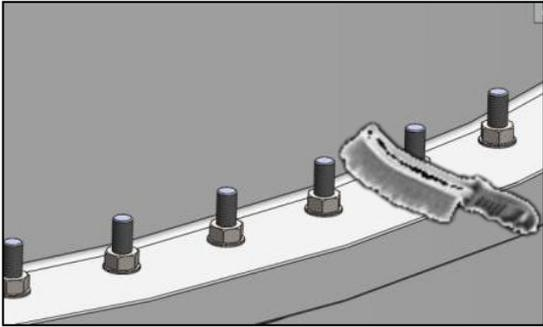
Before operating the tensioner, please clean the surface and thread of the bolt
