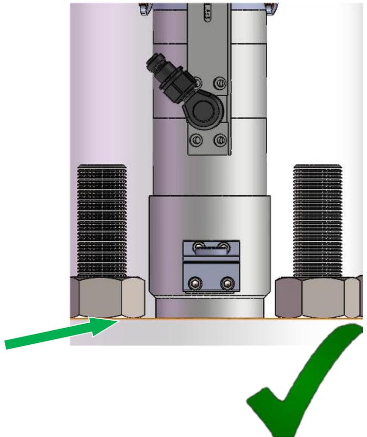
5. Screw the tensioner into the bolt with a manual torque wrench. Make sure that the gear sleeve and the nut are properly engaged.
