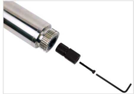
FIGURE 20 – Drive square removal
