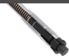
Turn fulcrum screw CCW direction to "UNLOCK" the wrench for torque setting; turn screw CW direction to "LOCK".
