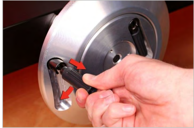
FIGURE 15 – Locking the Drive Wheel Handle
