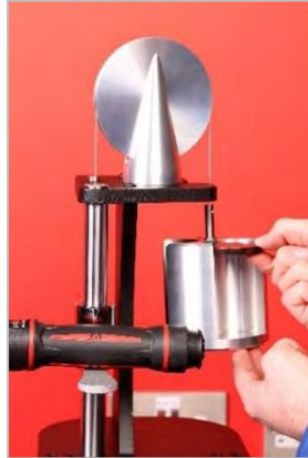
FIGURE 10 – Adding Weights to the Counter Balance Assembly
