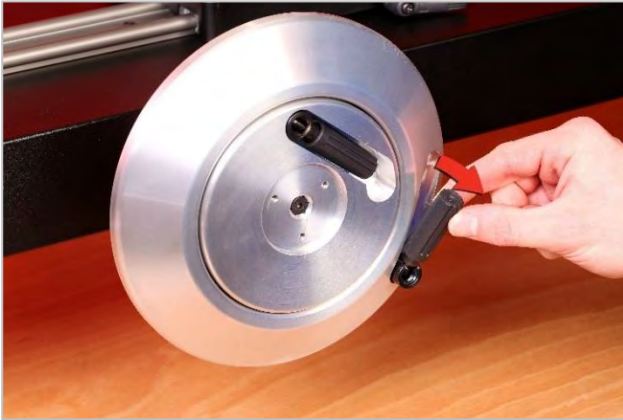
FIGURE 14 – Unlocking the Drive Wheel Handle
