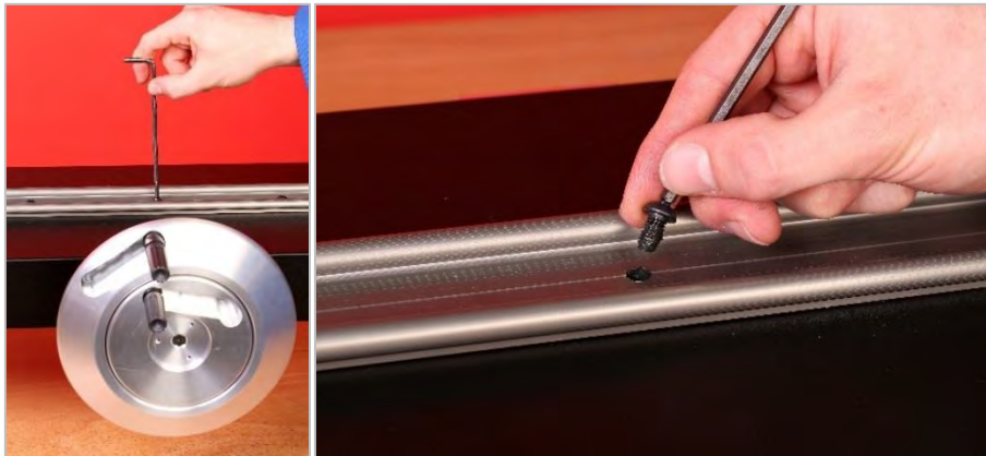
FIGURE 20 – Removing Button Head Cap Screw
