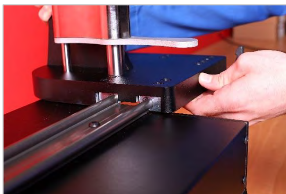
FIGURE 5 – Sliding the Counter Balance Reaction Assembly onto the Reaction Rail
