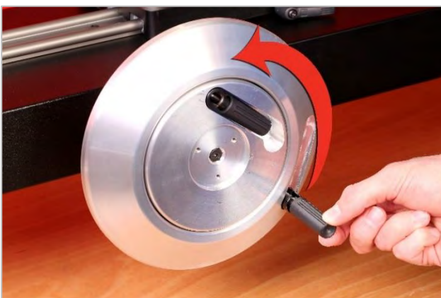
FIGURE 12 – Adjusting the TWC to Minimum Position
