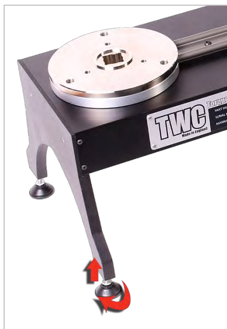
FIGURE 3 – Adjusting the TWC Feet
